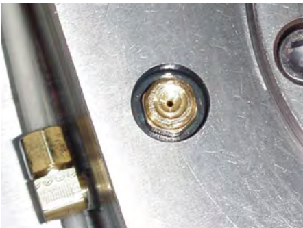
Magnetic Based Spray Assemblies Provides flexibility to locate the nozzles as required for each die. (pages 16, 18 and 19)
