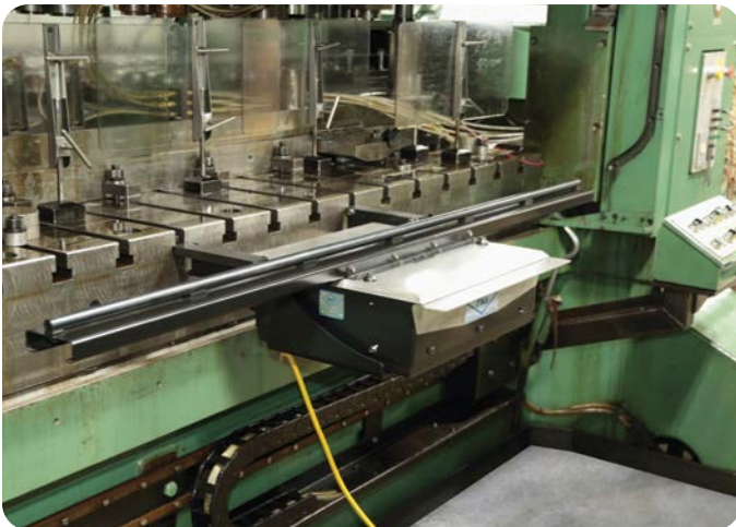
EGD-125 T-Slot Mounted with a 72" Standard Crossbar (trays are not shown)
