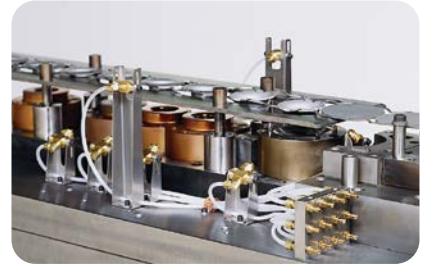
In-Die Spray Lubrication
