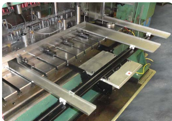
EGD-125 mounted in t-slots with 96" cross bar and 3 trays with Pax Tray Mounting Brackets
